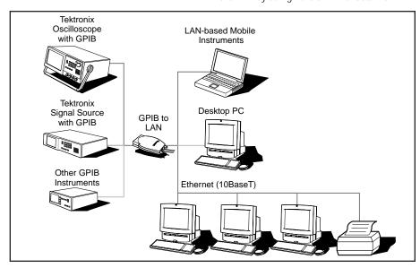
Several GPIB-networked instruments can be connected using the AD007 Adapter to LAN (Ethernet)-based computers and printers.
